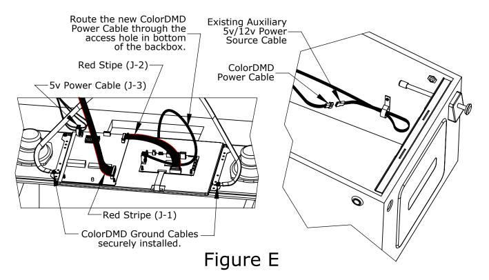
TIP Route the new ColorDMD Power Cable inside the cabinet along with other existing cables for a clean install.
